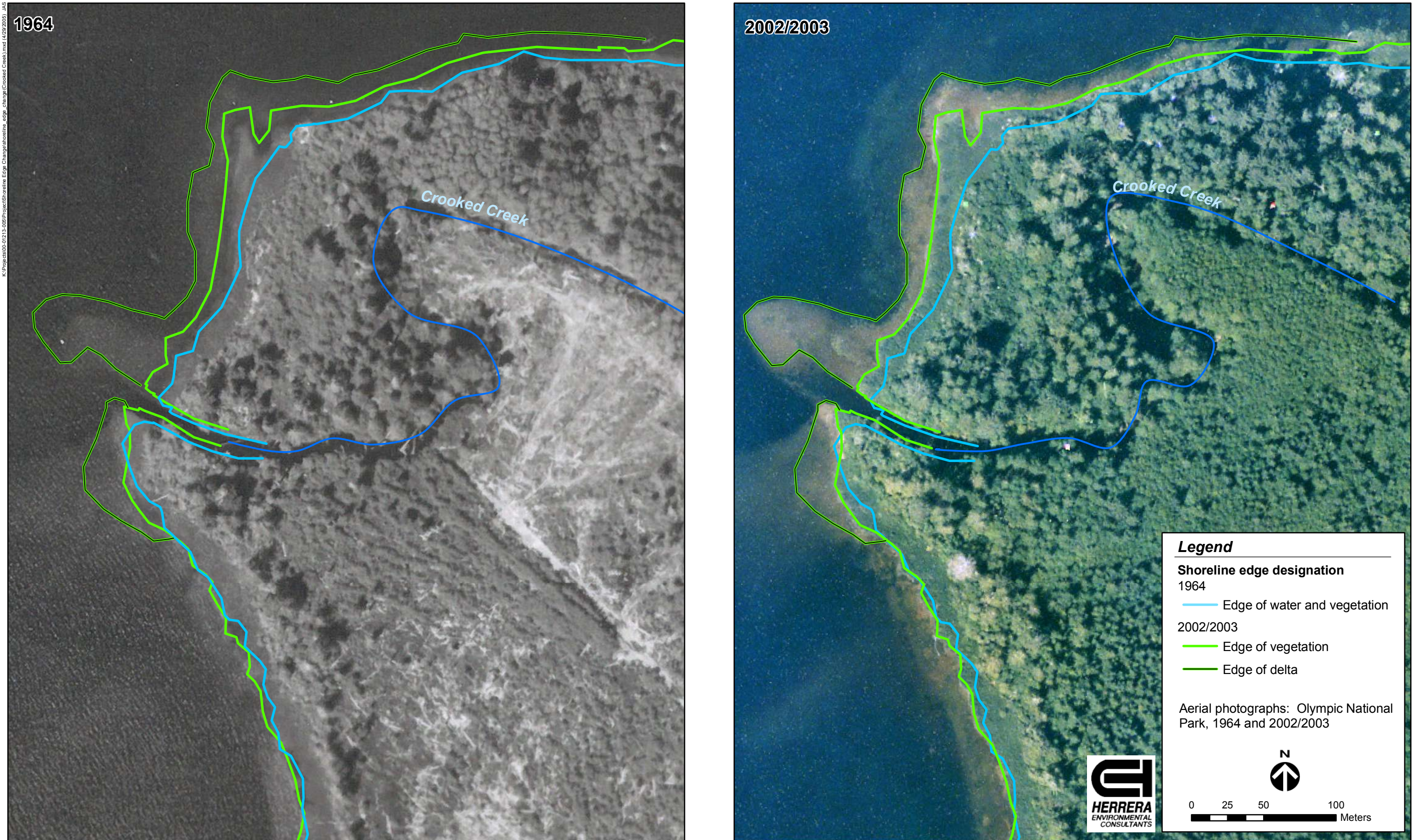
Figure 18. Shoreline changes and delta growth at the mouth of Crooked Creek between 1964 and 2002/2003, Lake Ozette, Washington .
